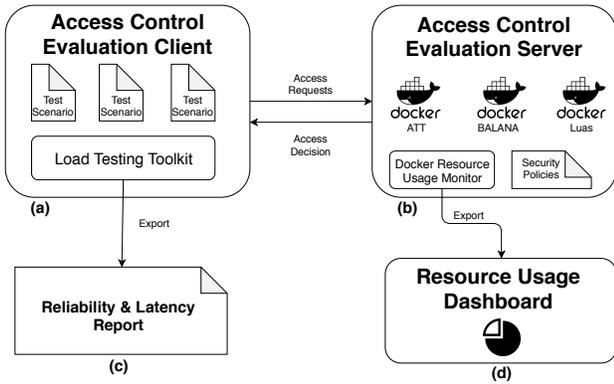
Fig. 1. System Diagram for XACML Evaluation Testbed. (a) is the access control client for sending access requests based based pre-defined test scenarios. (b) is the access control server which serves each PDP access control server via *Docker*. (c) is the aggregated report of reliability and latency, which is generated from (a). (d) is the dashboard to visualise matrices collected from (b)
