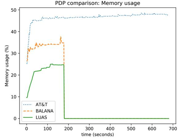
Fig. 2. Memory Usage % using data every 2 seconds from the Testbed Dashboard, for the 3 PDPs. Luas uses less memory during the experiment.
