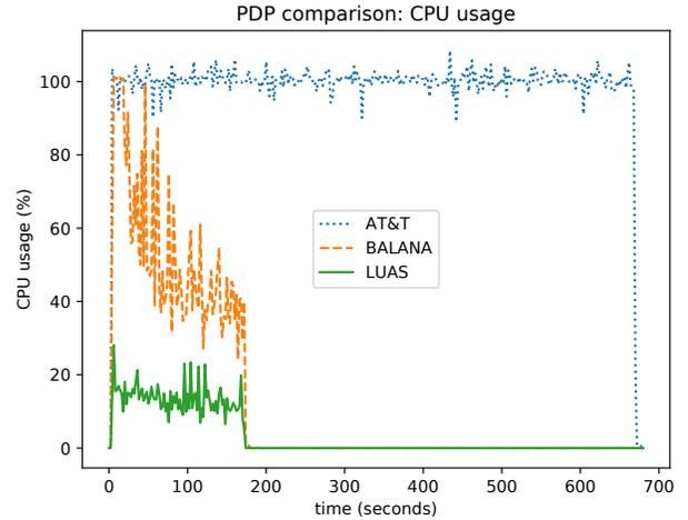
Fig. 3. CPU Usage % using data every 2 seconds from the Testbed Dashboard, for the 3 PDPs. Luas uses much less CPU during the experiment.
