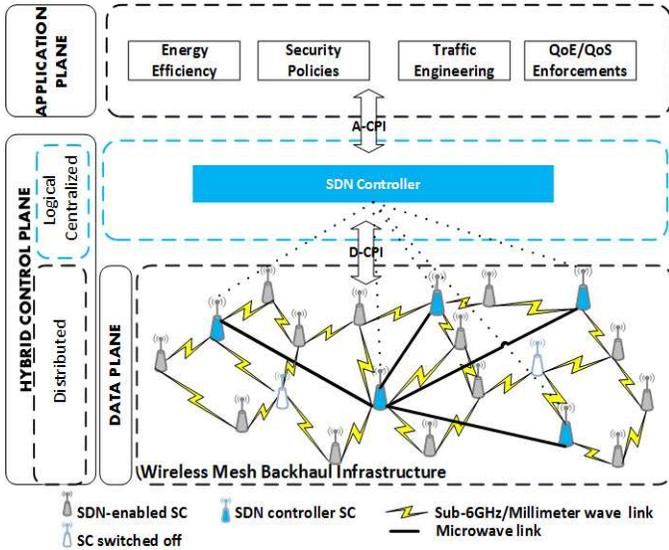
Fig. 1. The proposed service-based Hybrid SDN (hSDN) architecture.
