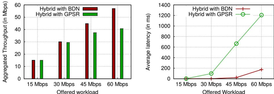
Fig. 3. Data plane performance of service-based hSDN model under SDN controller failure during a 40 minute period.
