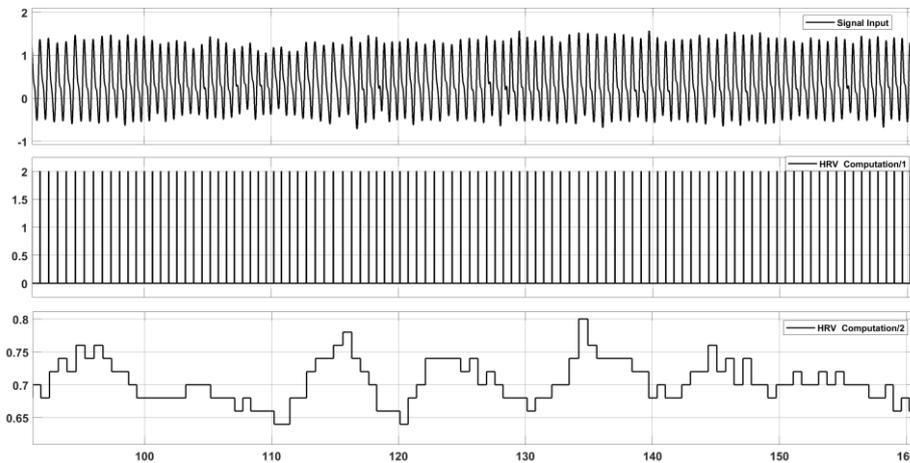
**Fig. 7.** Display output of the Simulink<sup>®</sup> system of a PPG signal of 160 seconds. The PPG input signal, peak detection and HRV estimation are represented in the first, second and third plot, respectively.
