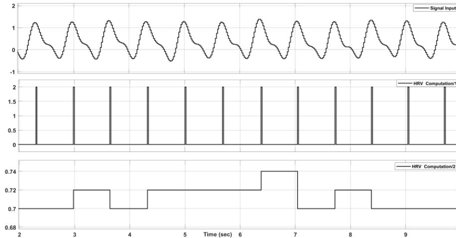
**Fig. 6.** Ten seconds display output of the Simulink<sup>®</sup> system. The PPG input signal, peak detection and HRV estimation are represented in the first, second and third plot, respectively.
