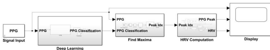
**Fig. 1.** Real-time HRV estimation system developed in Simulink<sup>®</sup>. This system is comprised by three main blocks: *Deep Learning*, *Find Peaks* and *HRV Computation*.
