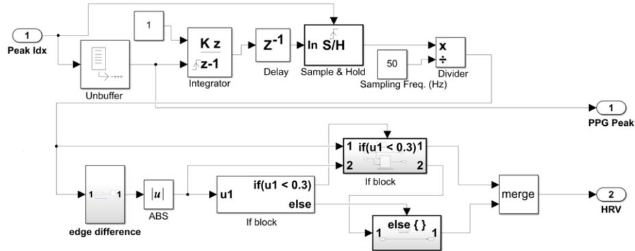
**Fig. 5.** *HRV Computation* block. From the peak index input, a sample distance between peaks is determined from which the HRV can be obtained. More details can be found in the text.
