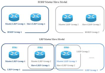
Fig. 3 Master/Slave Model HSRP vs. LRP
