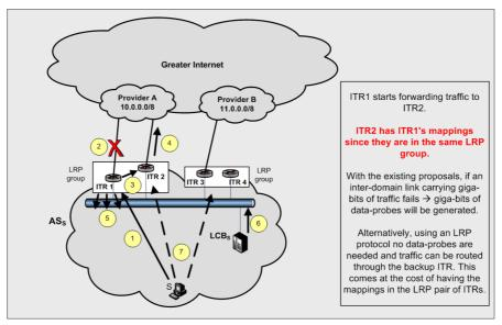
Fig. 4 LRP: Inter-domain link failure
