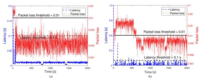
Fig. 2: Variation of KPIs observed over time using the testbed implementation: (a) N = 1, (b) N = 10.
