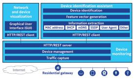
Fig. 1. Architecture of the IoT device identification assistant
