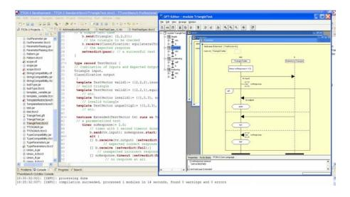
Fig. 3. A TTCN-3 Integrated Development Environment based on Eclipse
