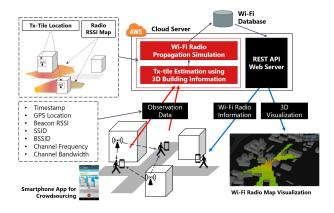
Fig. 2. System Architecture
