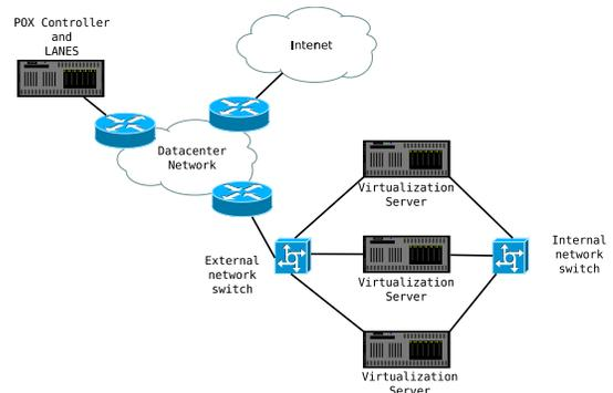
Fig. 3: Physical topology of the testing environment.
