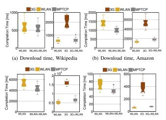
(c) Download time, Huffington Post (d) Packet delay, CBR video Figure 1. Download times for selected websites, and application packet delay for CBR video traffic, both over MPTCP in WLAN+WLAN (left of each pair) and **3G+WLAN** (right of each pair) (CORE emulation, with background traffic, see III-1). MPTCP with heterogeneous paths (**3G+WLAN**) underperforms single-path TCP on the best (WLAN) path.
