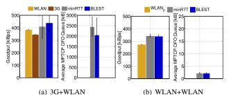
(a) 3G+WLAN (b) WLAN+WLAN Figure 8. **3G+WLAN** and **WLAN+WLAN** scenarios for bulk traffic with minRTT, BLEST and TCP on 3G and WLAN.
