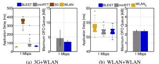
Figure 11. **3G+WLAN** and **WLAN+WLAN** scenarios for 1 Mbps CBR traffic with minRTT, BLEST and TCP on 3G and WLAN.
