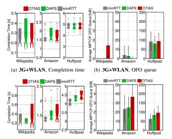
(c) **WLAN+WLAN**, Completion time(d) **WLAN+WLAN**, OFO queue Figure 4. Completion time and OFO queue for web traffic (Wikipedia, Amazon and Huffington Post) for DAPS, OTIAS and minRTT.
