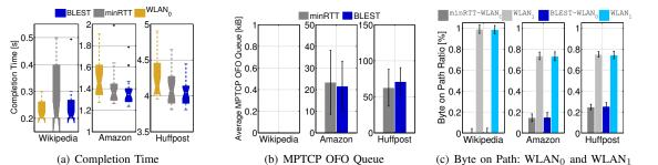
Figure 10. WLAN+WLAN for web traffic with Wikipedia, Amazon and Huffington Post with minRTT, BLEST and TCP on WLAN (WLAN0 and WLAN1).
