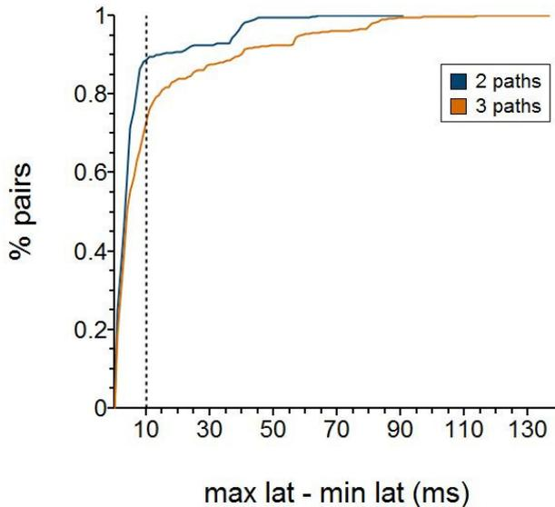
Fig. 9: For  $P = 2, 3$  and  $\Delta d$  we show the percentage of pairs that have a difference of latency between the IGP path and the worst path in the path set found by our algorithm at most  $\Delta d$ .
