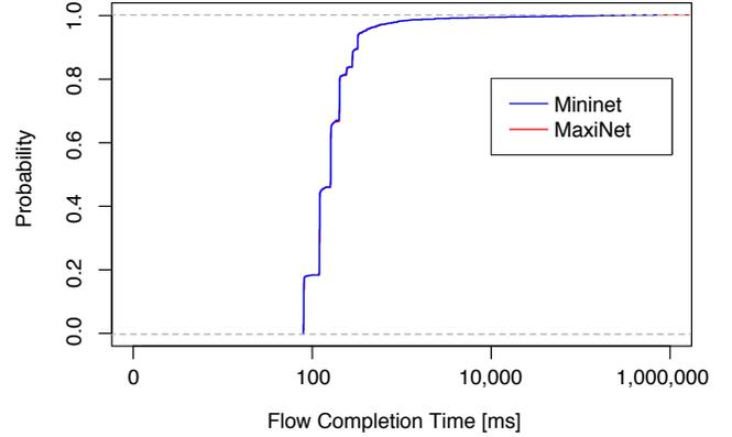
Fig. 10. Distribution of flow completion times between 300 servers emulated at a) one worker (Mininet), and b) four workers (MaxiNet) in a Clos-like network with a dilation factor of 200.
