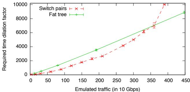
Fig. 6. Required dilation factor when emulating on a single physical machine. Confidence interval for a confidence level of 0.95.
