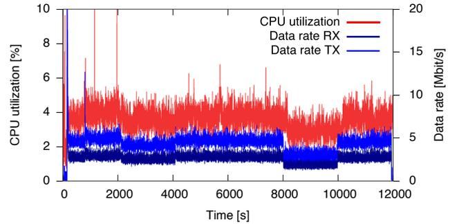
Fig. 12. CPU utilization and network usage of the OpenFlow controller over the course of the simulation.
