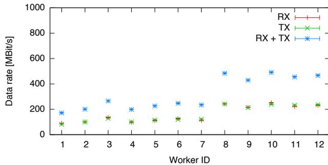
Fig. 14. Average network usage of the 12 workers during the large-scale experiment. Confidence intervals with confidence coefficient of 0.95 given.
