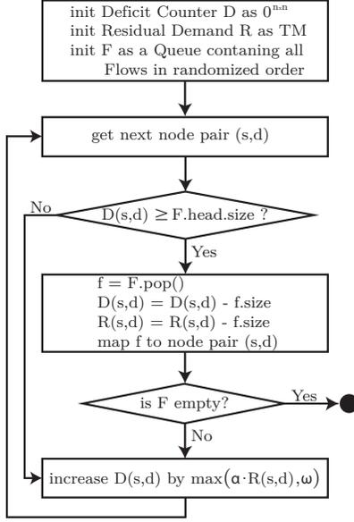
Fig. 3. Selecting s-d pairs for flows using Deficit Round Robin.
