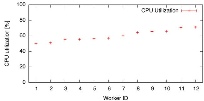
Fig. 13. Average CPU usage of the 12 workers during the large-scale experiment. Confidence intervals with confidence coefficient of 0.95 given.
