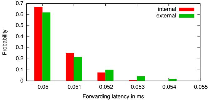
Fig. 8. Distribution of forwarding delays between nodes emulated at the same/different worker nodes.
