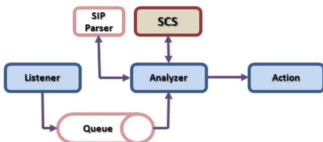
Fig. 2. Sensor Architecture
