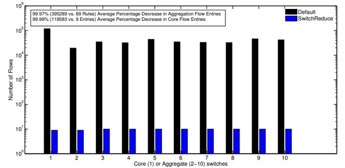
Fig. 6. Compression achieved by SwitchReduce on Aggregation/Core switches
