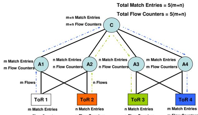
Fig. 1. Repetition of match entries and flow counters at every hop in the network
