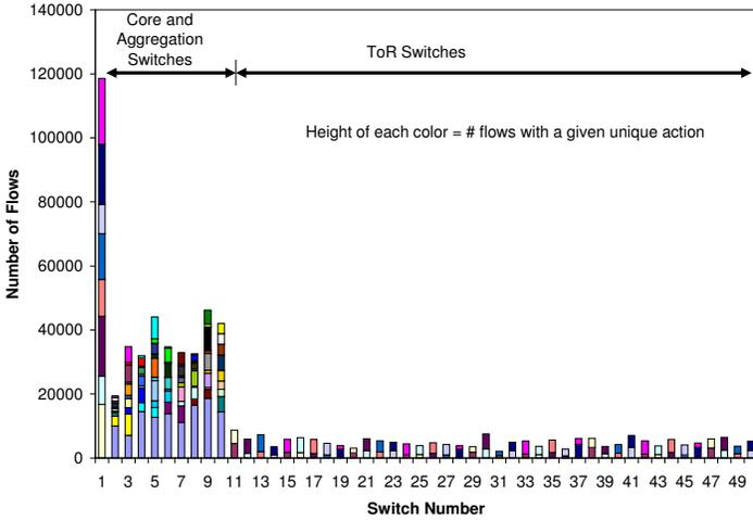
Fig. 4. Action overlap on Host ToRs and Aggregation/Core switches
