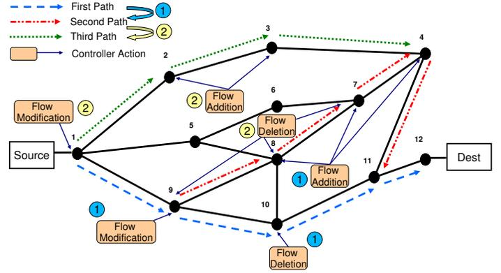
Fig. 10. Controller involvement in re-routing flows
