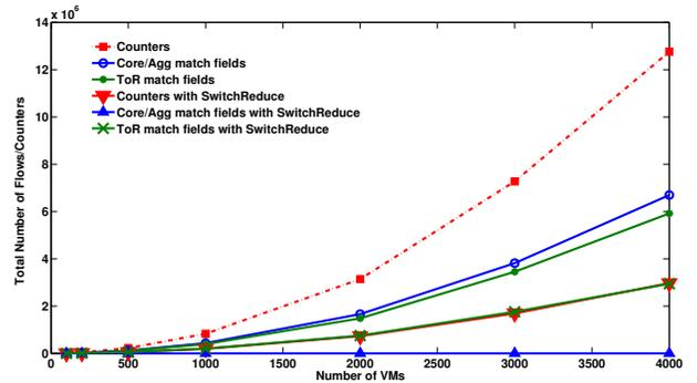
Fig. 8. Rate of increase of flow counters and match entries with VMs
