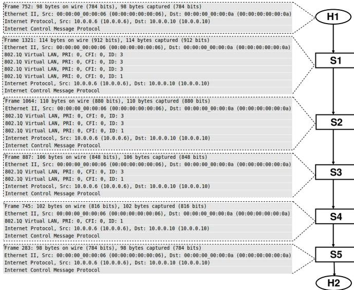
Fig. 3. Wireshark snapshot of a ping message from Host H1 to Host H2 - RouteHeader is [1,3,3,3]
