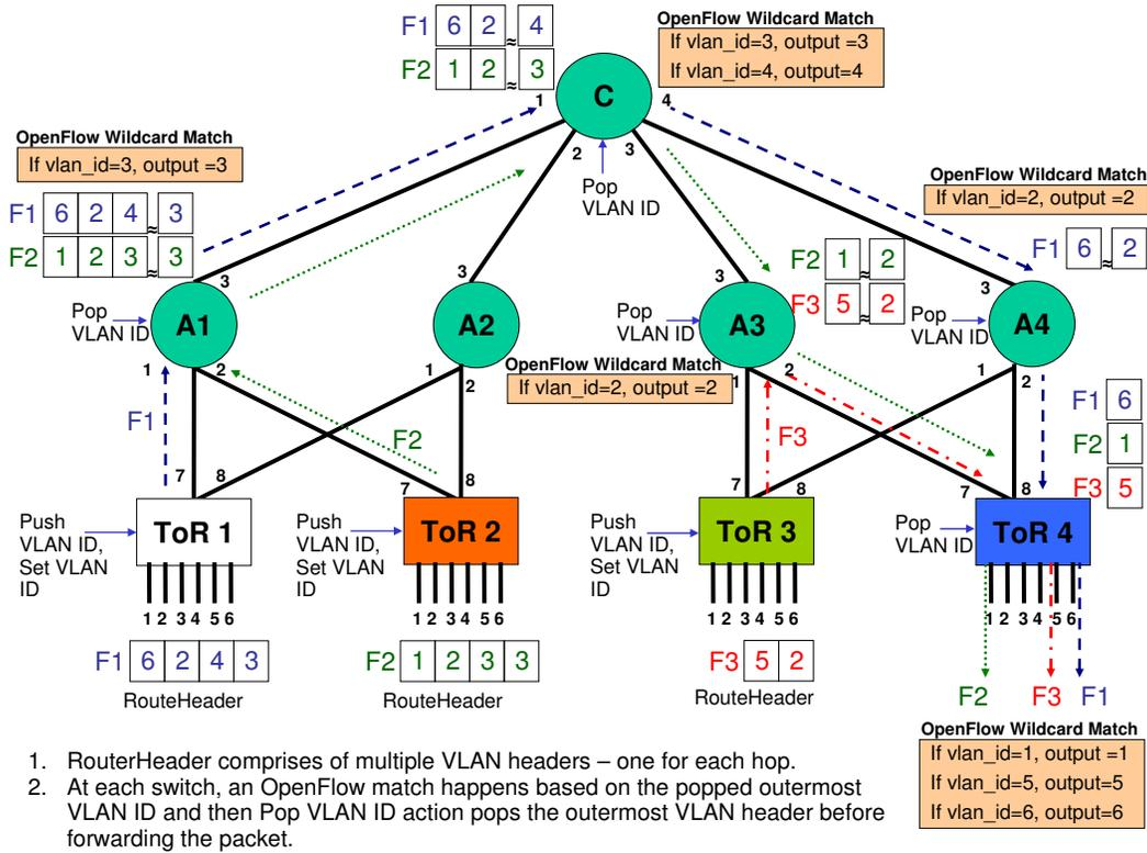
Fig. 2. RouteHeaders and use of Push VLAN ID and Pop VLAN ID operations in SwitchReduce
