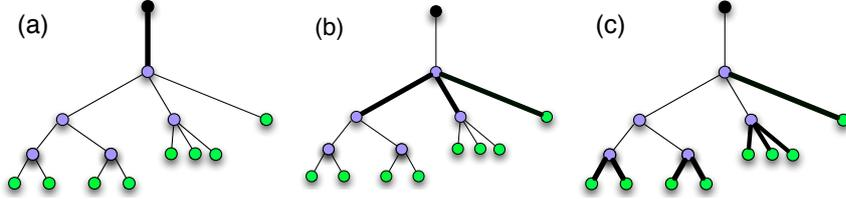
**Fig. 2.** Example of ambiguity in the locations of lossy links (bold), each of loss  $x$ . In each case, receiver vector  $\mathbf{y} = [x, \dots, x]^T$ , but the no. of lossy links varies - 1, 3, and 8.
