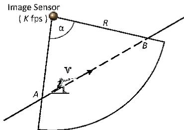
**Fig. 1.** Number of frames  $F$  produced by a single sensor node upon detection is  $F = K \frac{D_{AB}}{V}$  where  $K$ ,  $V$  and  $D_{AB}$  stands for the camera frame rate, target speed and pathlength respectively. The pathlength  $D_{AB}$ , in turn, depends on the sensing radius  $R$  and the FoV,  $\alpha$ .
