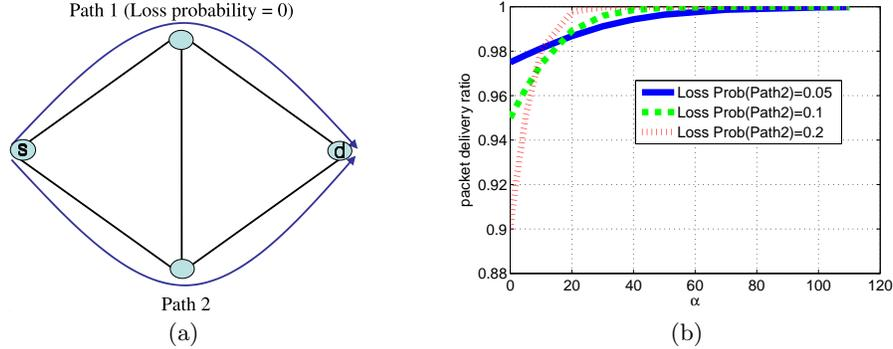
**Fig. 4.**  $\alpha$  versus Packet Delivery Ratio. The *link gain* parameter,  $\alpha$ , to achieve a certain packet delivery ratio depends on the loss probabilities of the paths.
