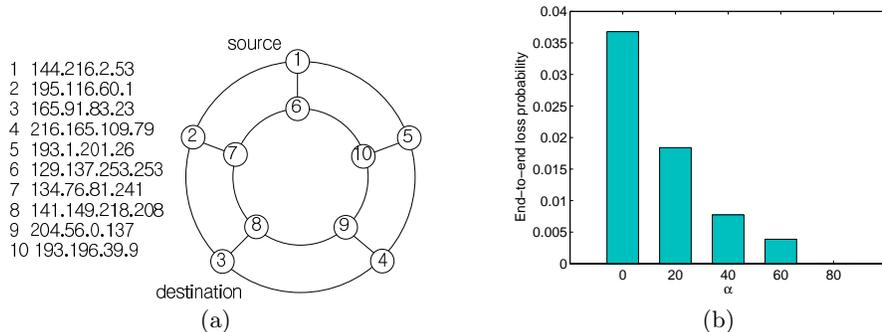
**Fig. 3.** Effect of *link gains* on end-to-end loss rates : (a) Hosts and topology used in the experiments. The links incident to node 8 usually have high loss rates, because node 8 is connected via DSL. (b) Number of lost packets with respect to 5 different  $\alpha$  values.
