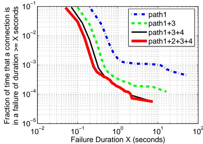
**Fig. 1.** An example result for a group. The Y-axis represents the fraction of time that the connection is in a failure of the duration  $\geq X$  seconds.
