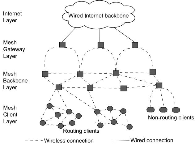
**Fig. 1.** Wireless Mesh Network architecture
