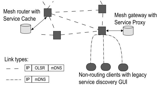
**Fig. 2.** Scenario A: service discovery support for non-routing clients
