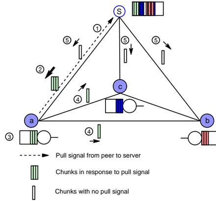
Fig. 2. Queue-based chunk scheduling example with four nodes
