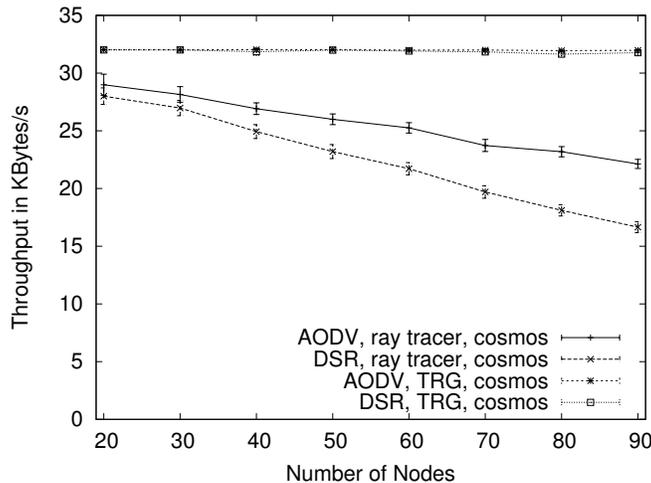
**Fig. 3.** Throughput comparison between AODV and DSR.
