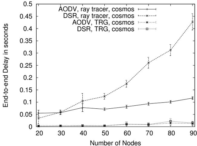
Fig. 4. Delay comparison between AODV and DSR.
