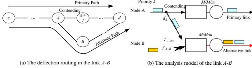
**Fig. 1.** The analytical model of the APDR scheme
