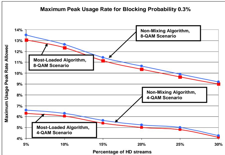
Fig. 6. Maximum Peak-Usage Rate Allowed vs. Percentage of HD streams using No-Mixing and Most-Loaded Algorithm for 4 and 8-QAM Scenarios
