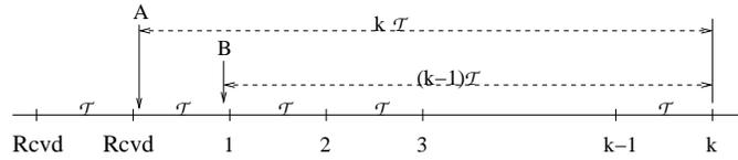
**Fig. 2.** Failure detection time for the non-cooperative approach
