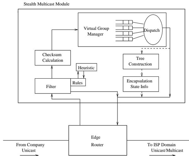
**Fig. 2.** Stealth multicast module - basic components
