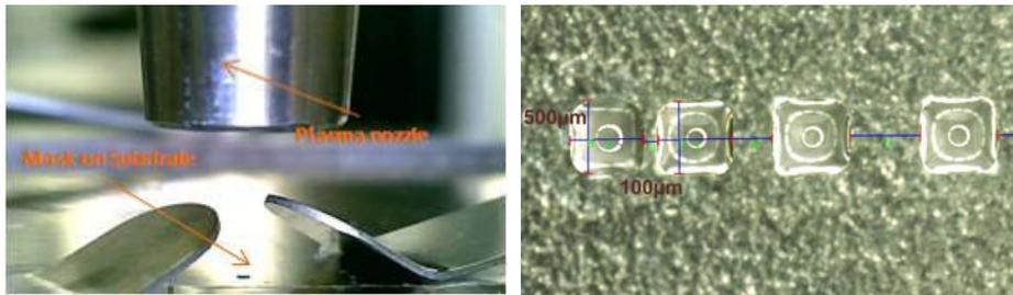
**Fig. 3.** Left: SMD-mask on polymer substrate and plasma nozzle above. Right: Droplets on functionalized surface with 500 $\mu$ m edge length and minimal spacing of 100 $\mu$ m
