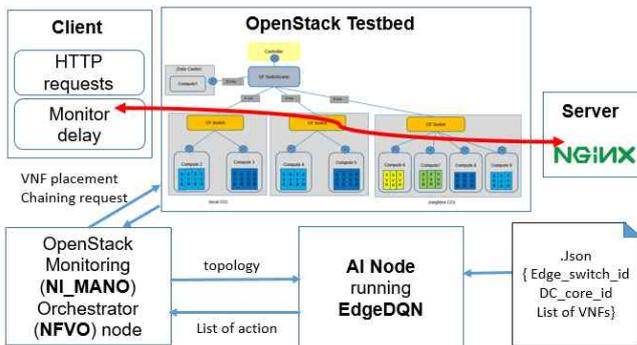
Figure 7: Integrating EdgeDQN with OpenStack
