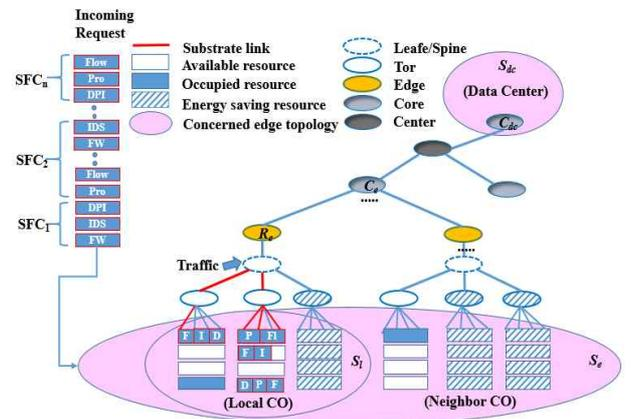
Fig 1: Possible placement operation of SFCs with minimum substrate link delay and maximum resource utilization on an Edge cloud environment.
