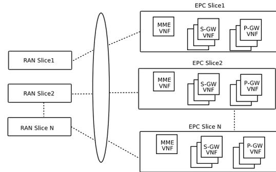
Fig. 2. Network Slicing System Model.
