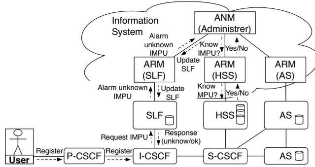
Fig. 2. The case of a SIP-based VoIP service
